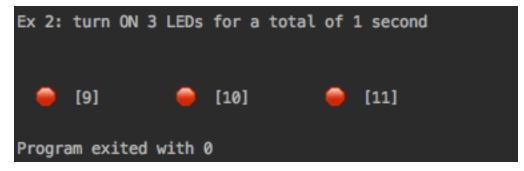
**Technical explanation:** the script is supposed to display the LEDs turning ON and OFF always on the same line. That is, when a line of LEDs is displayed, the script goes to the beginning of the line to display the next state of LEDs by printing over the previous LEDs.
